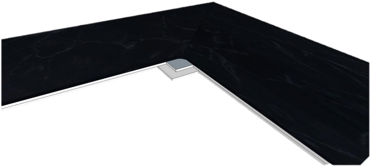
Figure 14. Movement miter joint topside utilizing the “Interlocking Corner Block Method”
